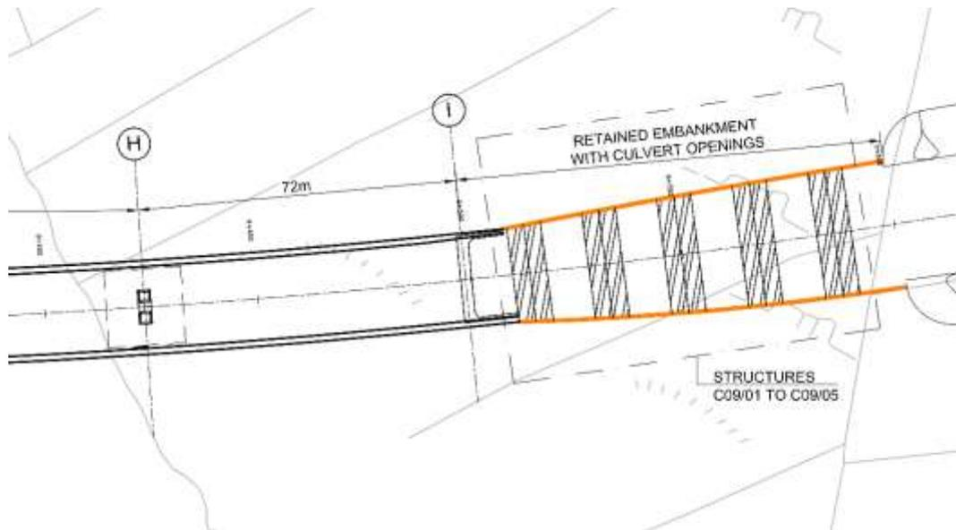
**Figure 2.12: Elevation of Retained Embankment Tie-in**
