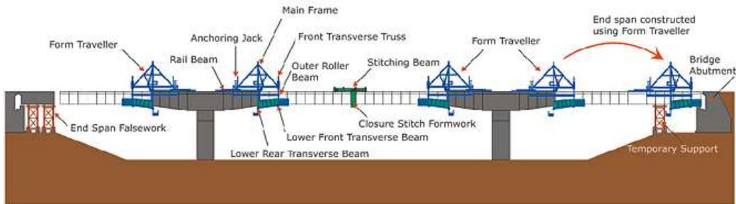
**Figure 2.10: Travelling Formwork**
